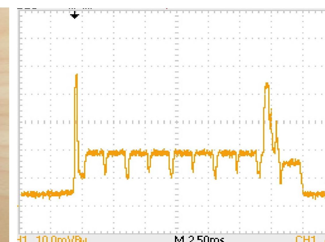
Figure 2 Current Consumption for Microduino on Oscilloscope
